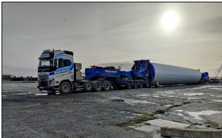
Figure 2-5: Bogie type tower transporter
