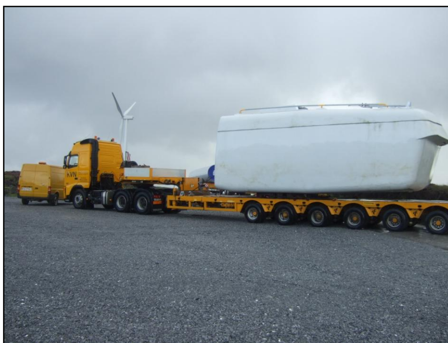
Figure 2-6: Semi low-loader type tower transporter
