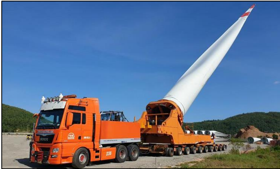
Figure 2-3: Blade lifter trailer with blade tilted to 60° to the horizontal
