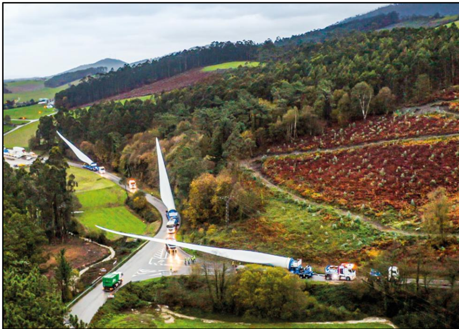
Figure 2-4: Blade lifter trailers in convoy transitioning from tilted to lowered to avoid overhead line
